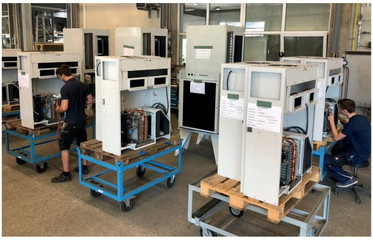
In the main plant in Amtzell, Germany all products made by FrigorTec GmbH are developed, constructed and produced. Every device passes a quality inspection with test runs before delivery. FrigorTec solutions are sold in over 84 countries through our worldwide distribution network.
