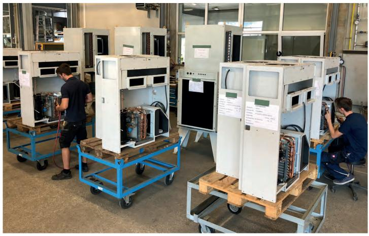
In the main plant in Amtzell, Germany all products made by FrigorTec GmbH are developed, constructed and produced. Every device passes a quality inspection with test runs before delivery. FrigorTec solutions are sold in over 100 countries through our worldwide distribution network.
