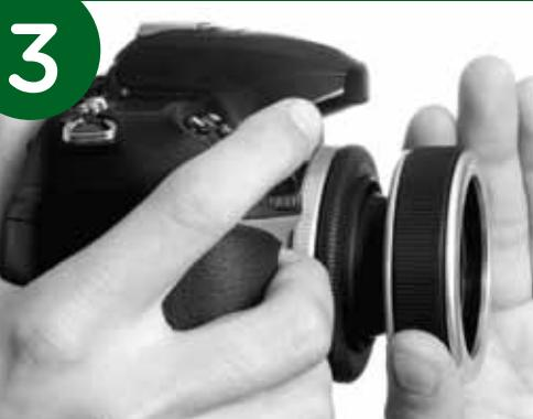
**EN** Point the Composer straight ahead and focus by turning the Focus Ring to bring the center of the image in focus.
