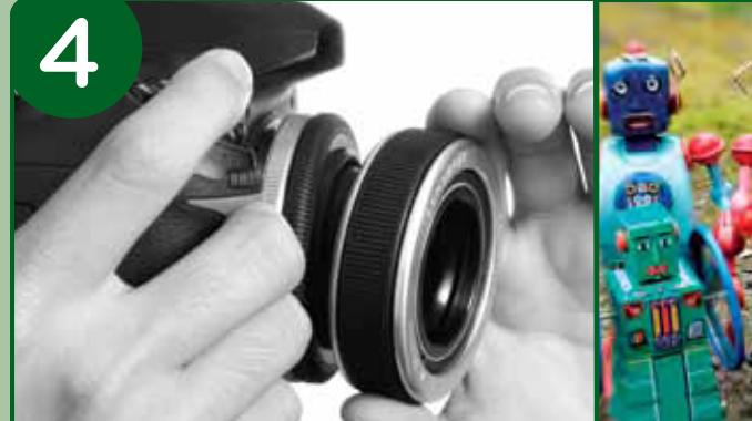
**EN** Tilt the Composer in the direction you want your Sweet Spot of sharp focus to move and then re-adjust the focus with the Focus Ring. Try tilting in small amounts until you get a feel for how much you need to tilt the lens to place the Sweet Spot where you want it. You are now ready to shoot!
