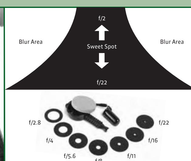
**EN** You can remove the Aperture Disk by touching the tip of the Aperture Tool to the disk and slowly lifting it out. Drop in a new disk. The size of the Sweet Spot is controlled by your aperture. The larger the aperture opening the smaller the Sweet Spot.
