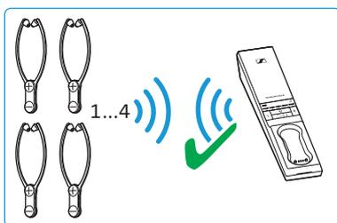
You can simultaneously use up to 4 paired stethoset receivers with your transmitter. All other paired and switched-on receivers cannot connect to the transmitter.
