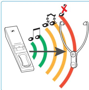
The range of the transmitter largely depends on environmental conditions such as wall thickness, wall composition etc. If you, and therefore the stethoset receiver, leave the range of the transmitter, the audio drops out occasionally at first before the connection breaks down completely. You hear alerts in the stethoset receiver.
