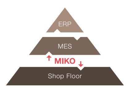
MIKO is the real-time data interface between MES and the wire processing machines.
