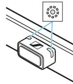
If audio encoding via the aptX codec is active, the status LEDs on the dongle housing light up pink.
