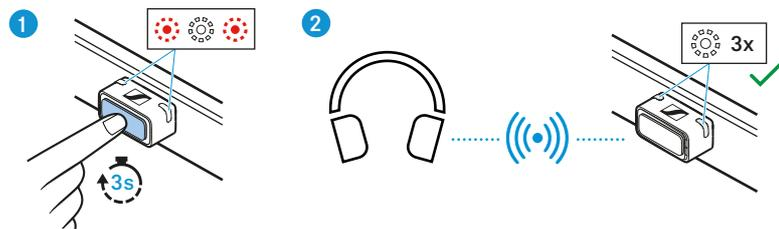
As soon as the dongle is paired with a pair of Bluetooth headphones, the status LEDs on the dongle housing flash white 3x.
