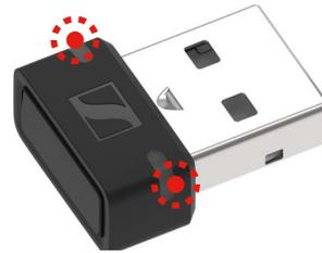
The two status LEDs on the dongle housing indicate the operating state of the dongle:
