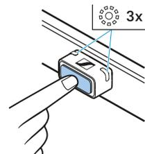
During the connection attempt, the status LEDs on the dongle housing repeatedly flash white 3x. The connection process can take up to 20 seconds.
