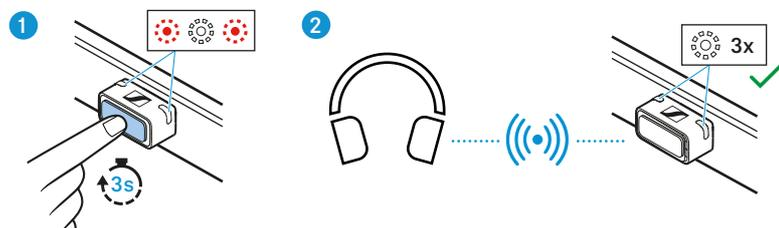
As soon as the dongle is paired with a pair of Bluetooth headphones, the status LEDs on the dongle housing flash white 3x.
