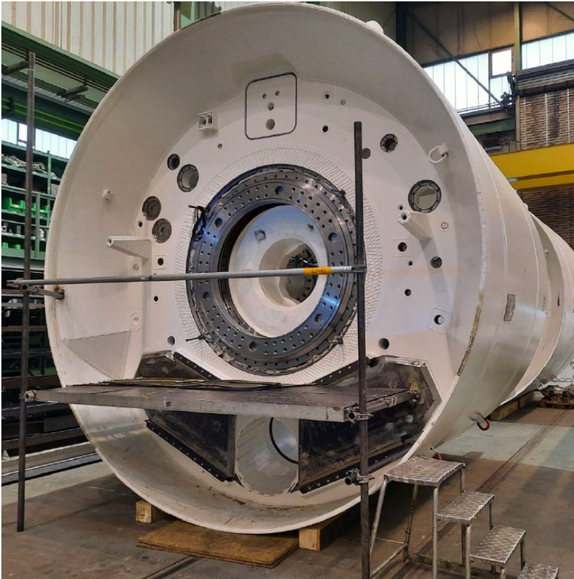
Tunnel Boring Machine Front Shield
