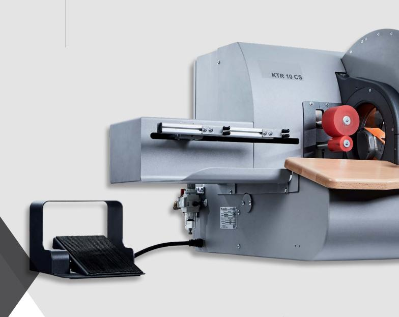
High precision from the start: Linear guidance ensures exact overlapping, even with short sections.
