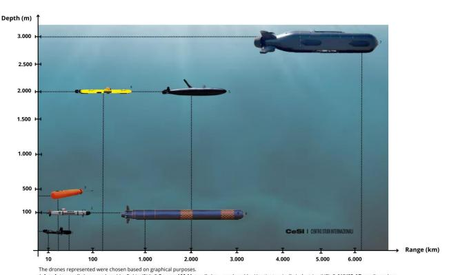
1 Amulete, small class, produced by Rubin (RU); 2 Remus 100 M, small class, produced by Huntington Igalls Industries (US); 3 AUV62-AT, medium class, produit de SAAB (SE); 4 Gavia, medium class, produced by Teledyne Marine (US); 5 Spearthooth, large class, produced by C2 Robotics (AU); 6 Haeil, large class, (RPDC); 7 Orca, Extra Large class, produced by Boeing (US).
