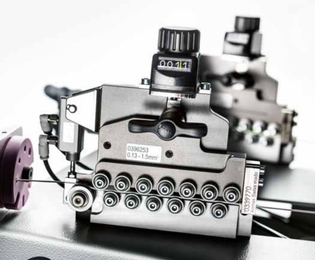
Straightener unit pneumatic with wire diameter display recommended for: 0.13–1.5 mm 2 .
