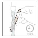
**2** Wait 1 minute. The number of squares on the test strip that turn red indicate the water hardness.
