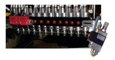
Valco Melton offers a gluing system consisting of a bank of non-contact valves that apply glue dots. Easy to integrate into machine, this solution avoids the need to run the product again for the second gluing application or to have a 90 degree turning attachment on your folder-gluer.
