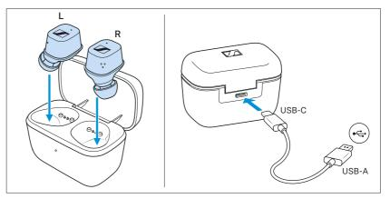
Upon delivery, the rechargeable batteries of the earbuds and the charging case are in sleep mode and have to be woken up by connecting them to a power source once.
