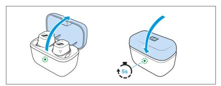
If you open the lid of the charging case and no USB cable is connected, the LED of the charging case displays the battery charge status or the charging process of the earbuds. If you close the lid of the charging case, the LED will go off after 5 seconds.
