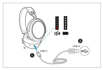
Connect the USB-C connector of the charging cable to the USB socket of the headphones. 2. Connect the USB-A connector to a corresponding socket of a USB power source (to be ordered separately). Make sure that the USB power source is connected to the power supply system. The charging process of the headphones begins. The LED display indicates the charge status.
