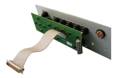
EAO provides a complete, custom front panel package for the HMI control system with Series 71 push button and Series 84 shallow back-of-panel E-Stops.
