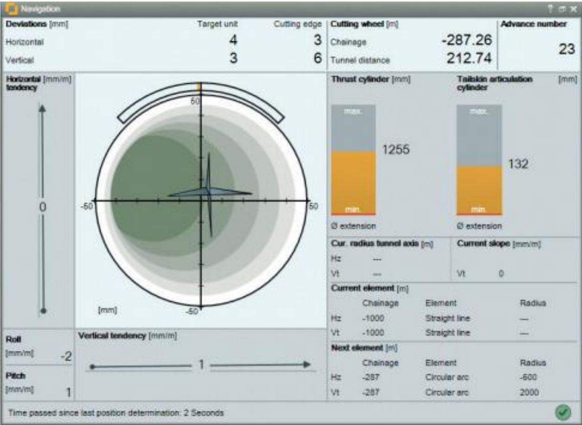
TBM orientation adjusted to target position based on preset tunnel alignment coordinates
