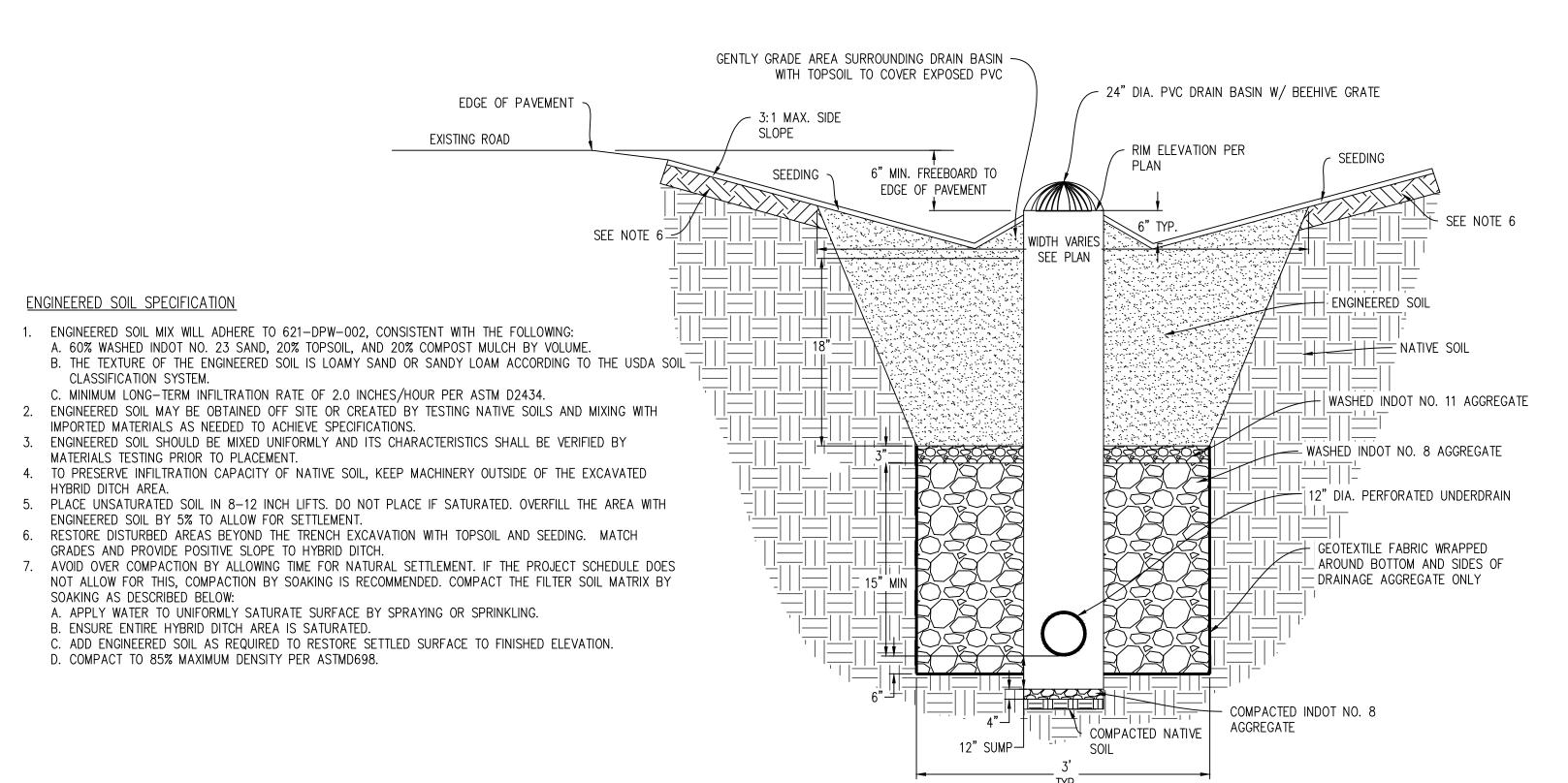
HYBRID DITCH TYPICAL SECTION > 5' DEPTH
