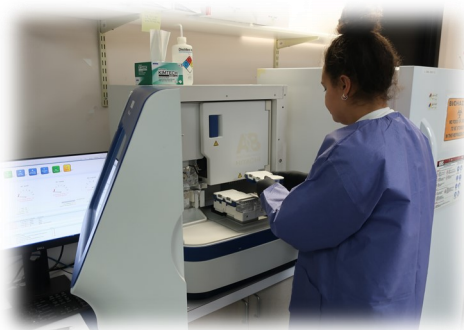
Forensic Scientist loading DNA samples on a genetic analyzer.
