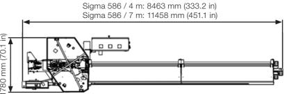
Height with closed cover: 1,985 mm (78.1 in) Height with cover completely open (maximum opening): 2,965 mm (116.7 in)
