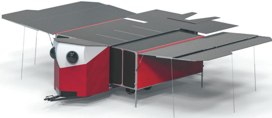
The panels of the Solar Butterfly make it possible to produce up to 170 kWh of solar energy a day, which will allow it to travel up to 300 km daily.
