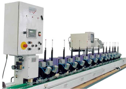
Placement machinery for IDC terminals
