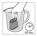
5 Immerse the filter upside down in a jug with cold water and shake/press it.
