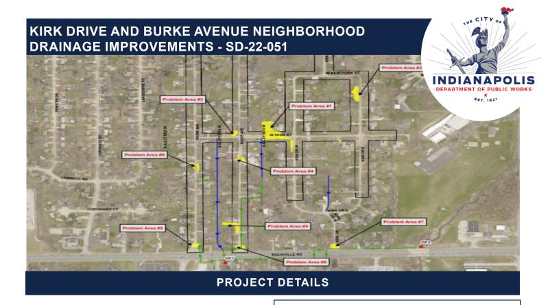
This project includes improvements to address standing water issues on Kirk Drive to Richie Avenue and from Rockville Road to Lockerbie Drive. Improvements will include hybrid ditches and storm sewers with street resurfacing. Work is expected to begin in late Fall 2022 through Fall 2023. Learn more at <a href="mailto:indy.gov/dpw">indy.gov/dpw</a>.
