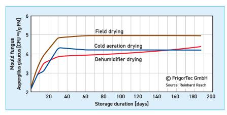
4 The difference between various drying methods on the development of the mould fungus Aspergillus glaucus (2)
