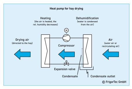
12 Heat pump process for air dehumidification
