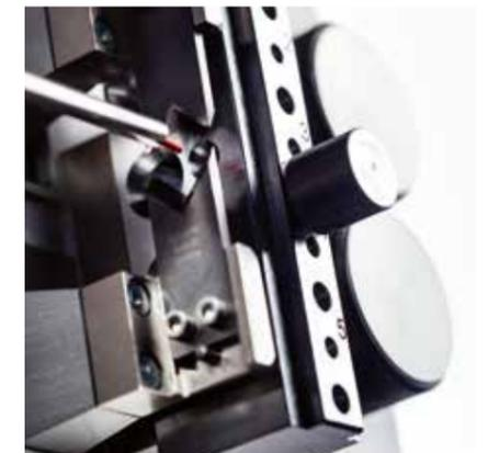
Blade head with 8-hole wire feeding system.
