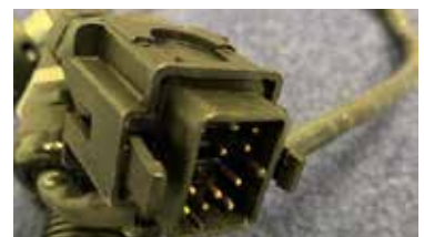
Quick Lock clamp on electrical connection
