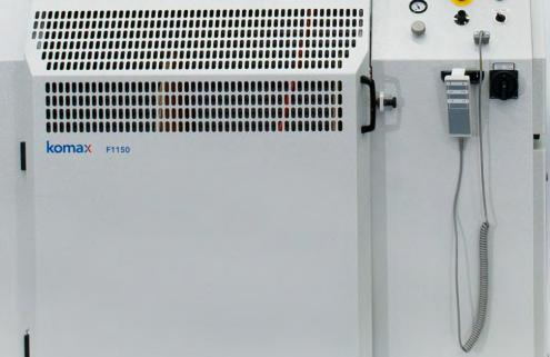
This automatic, low tension wire feed system, F1150 enables the processing of both thin, flexible strands and thicker, tension-sensitive wires such as coaxial cables.
