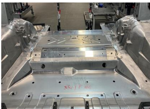
Rear Floor Assembly – Cast Aluminum
