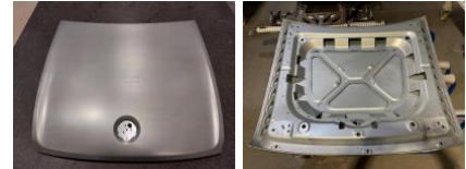
Hood Panel Assembly – Stamped Steel
