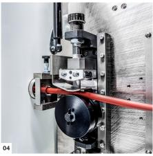
01 Heavy-duty wire straightener 02 Easy guide changes 03 Networking via WPCS protocol 04 Available wire slitting option
