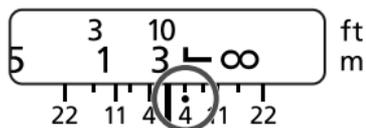
The infrared index corrects the focus setting when using monochrome infrared film. Focus on the subject manually, then adjust the distance setting by moving the focusing ring to the corresponding infrared index mark.
