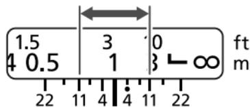
The depth of field is the distance in front of and behind the plane of focus on the subject that appears sharp. The depth of field is indicated by the area between the depth-of-field scale lines below the distance scale.
