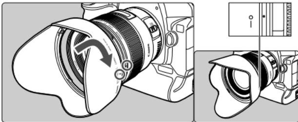
The EW-83K hood can keep unwanted light out of the lens, and also protects the lens from rain, snow, and dust.
