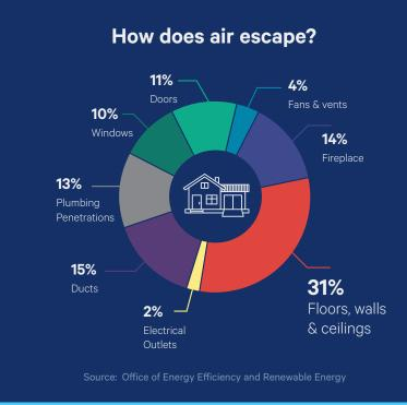
Nearly **one third** of air infiltrates through the openings in ceilings, walls and floors in a home with fiberglass insulation.
