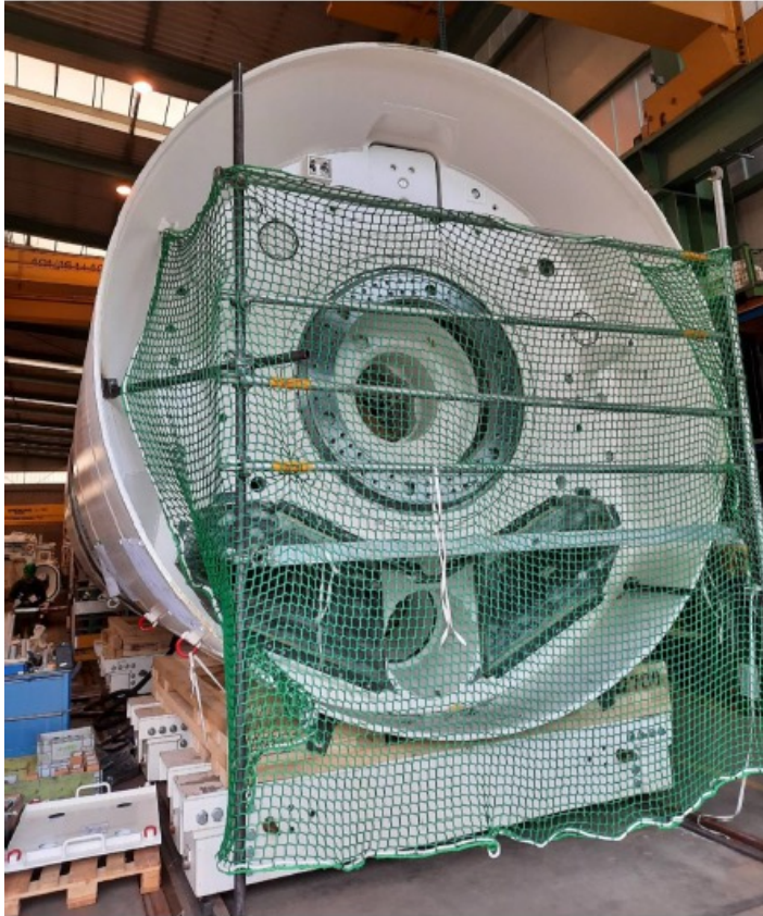
Tunnel Boring Machine Front Shield
