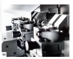
The line laser makes the positioning easier. 02 No reclamping of the sample necessary. 03
