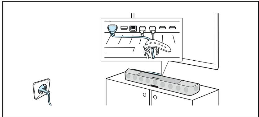
Connect the AMBEO Soundbar | Max to the power supply system - the AMBEO Soundbar | Max comes to life and guides you through the initial switch-on process (> 30).
