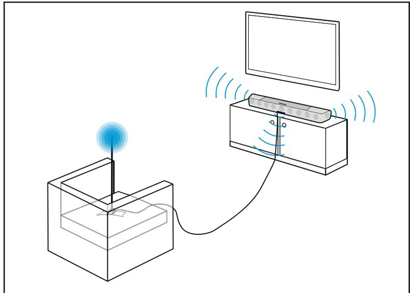
For an optimum spatial sound experience, the AMBEO Soundbar | Max must perform a room calibration. Connect the microphone for the room calibration and start the calibration. The calibration takes only a few minutes and leads to the best possible 3D spatial sound (> 31).
