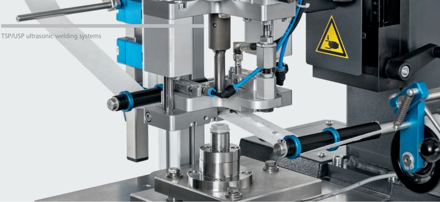
Gentle cutting and welding of a filter membrane in one work step (torsional)
