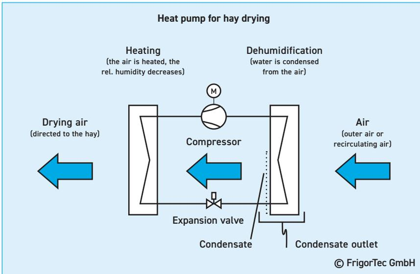
12 Heat pump process for air dehumidification
