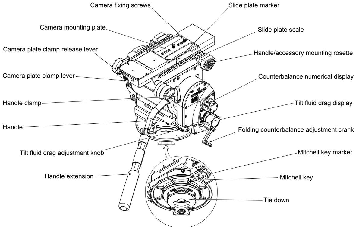
The 2575D pan and tilt head embodies a patented sinusoidal counterbalance mechanism for true and accurate balance; stepless drag assemblies for ultra-smooth pan and tilt motions; and an adjustable camera mounting plate.
