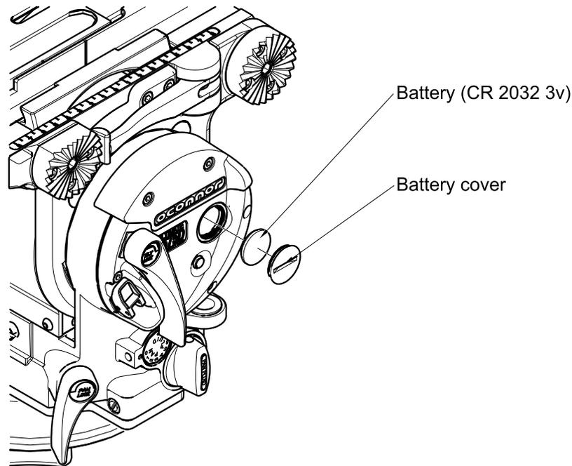
1. If required, rotate the tilt lock lever to assess the battery cover.
