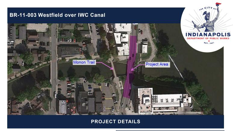
This project will replace the existing bridge over the Canal at Westfield Blvd. with a new single-span threesided arch bridge, railings and a sidewalk. The existing concrete bridge base will remain intact. The work will also repair and stabilize the northwest canal bank. Construction should begin in Winter 2022 with completion expected in Summer 2023. This project is coordinating with the Broad Ripple Avenue closure to ensure Broad Ripple remains accessible throughout each project.
