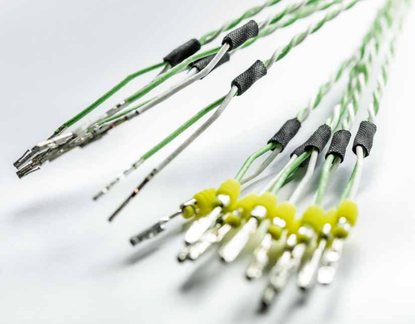
Taped unshielded twisted pairs (UTP) that fulfill OEM quality requirements.
