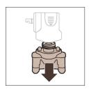
Disassemble the internal cappuccinatore by pulling the bottom part off the top part.
