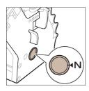
Before you slide the brew group back into the machine, make sure it is in the correct position.
