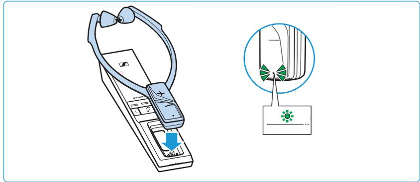
**i** If you place the stethoset receiver into the transmitter's charging compartment at the very beginning of the restore procedure, the factory settings of the transmitter and the receiver are restored simultaneously.
