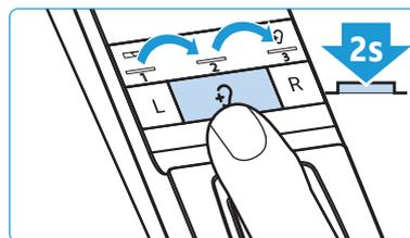
5. Test which of the hearing profiles (1, 2 or 3) gives you the best sound quality and helps you to hear best. Your individual hearing profile is adjusted and saved on the stethoset receiver.
