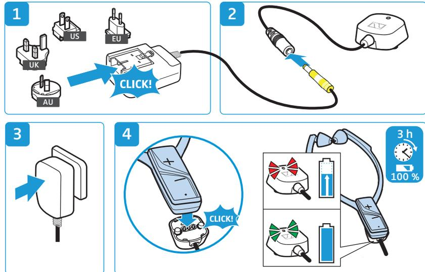
**i** You can also use the stethoset receiver during charging. Note, however, that the receiver can get slightly warm during charging. The charge status of the rechargeable battery is displayed on the transmitter (see page 15).
