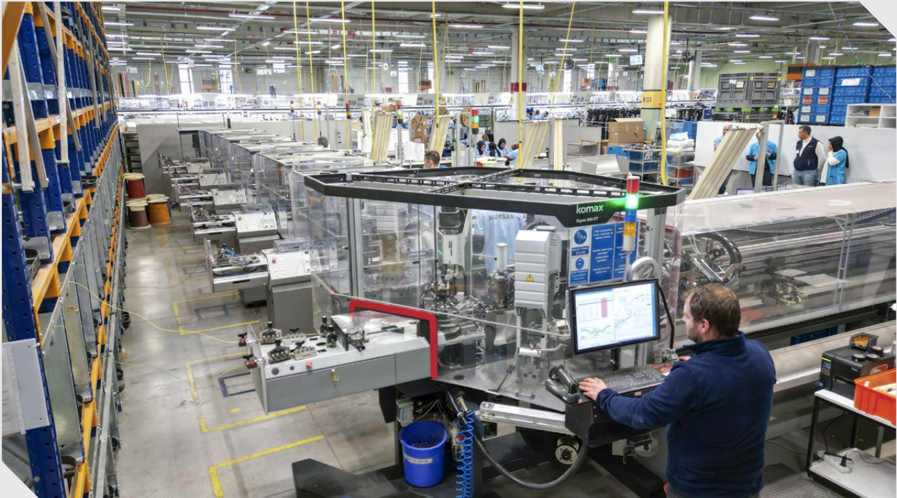
The biggest manufacturing site, Nursan's "Plant 1" in Tavşanlı, İstanbul, Türkiye, produces wire harnesses for up to 750 000 vehicles each year. Among the machines it uses to do this are Sigma 688 twisting machines, Komax's Alpha series crimp-to-crimp-machines, and the CrimpCenter from Schleuniger.
