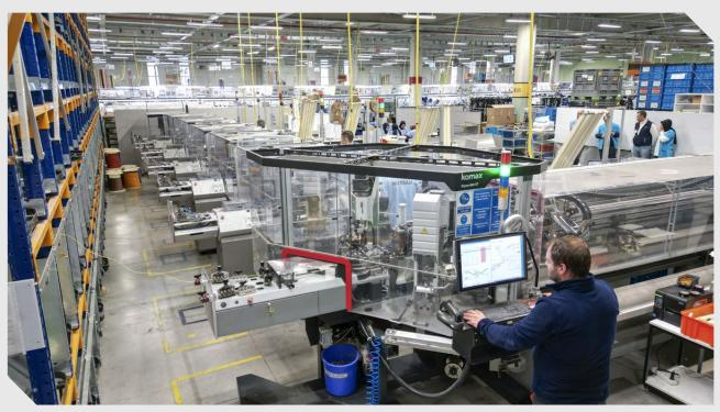
The biggest manufacturing site, Nursan's "Plant 1" in Tavşanlı, Istanbul, Türkiye, produces wire harnesses for up to 750000 vehicles each year. Among the machines it uses to do this are Sigma 688 twisting machines, Komax's Alpha series crimp-to-crimp-machines, and the CrimpCenter from Schleuniger.
