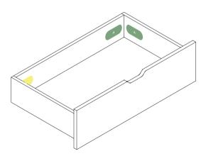
Pull out the bottom-most drawer tracks from the dresser as far as they'll go. Disengage the orange pin at the front of each track by pulling the trigger inward. The pins should be flush with the inside of the track before placing the drawer.
