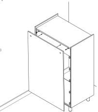
Place the dresser in its final position, and attach the anti-tip cables to their counterparts on the wall, following the instructions from Step 2.
