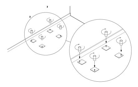
Using two thumbscrews for each corner, screw the leg and plate assemblies into the four corners of the base panel, with the leg in the outermost corner.
