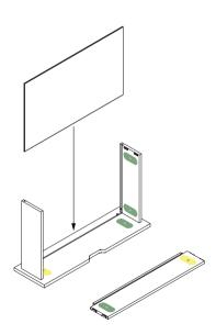
Finally, attach the back of the drawer by lining up the yellow (B) and green (A) stickers with the stickers on the drawer sides, making sure the groove at the bottom creates a continual line between the back and sides.
