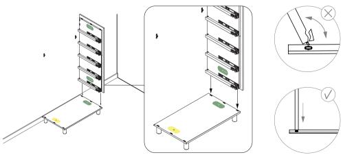
While someone holds the right wall upright, attach the left wall to the base panel by lining up the yellow (B) stickers, with the "Top B" sticker at the top. Just like the other wall, there are six clips: three on the edge of the base panel, and three on the edge of the wall. Align these clips, and press them together until you hear a click.
