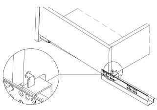
Once that's in place, lower the front of the drawer onto the track. Here, there are two pins: one gray and one orange. The gray pin will fit into the bottom edge of the drawer. The orange pin fits into the inside edge of
