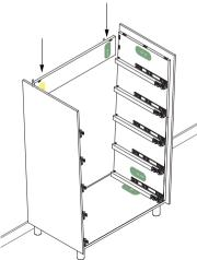
Attach the top panel to the side walls by aligning the yellow (B) and green (A) stickers, and clicking down into place at all connection points. Push or pull the top panel towards the back of the dresser to lock the clips.
