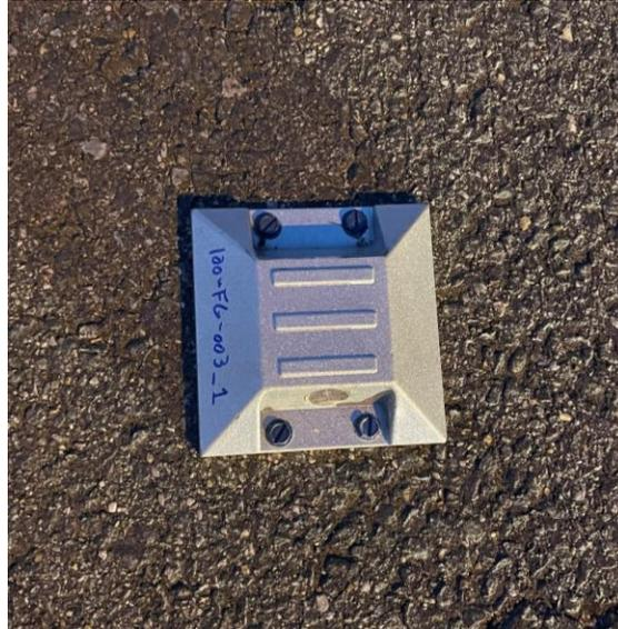
**Ground Monitoring Points** are passive, surface mounted devices used to survey the ground surface before, during, and after tunnel construction.
