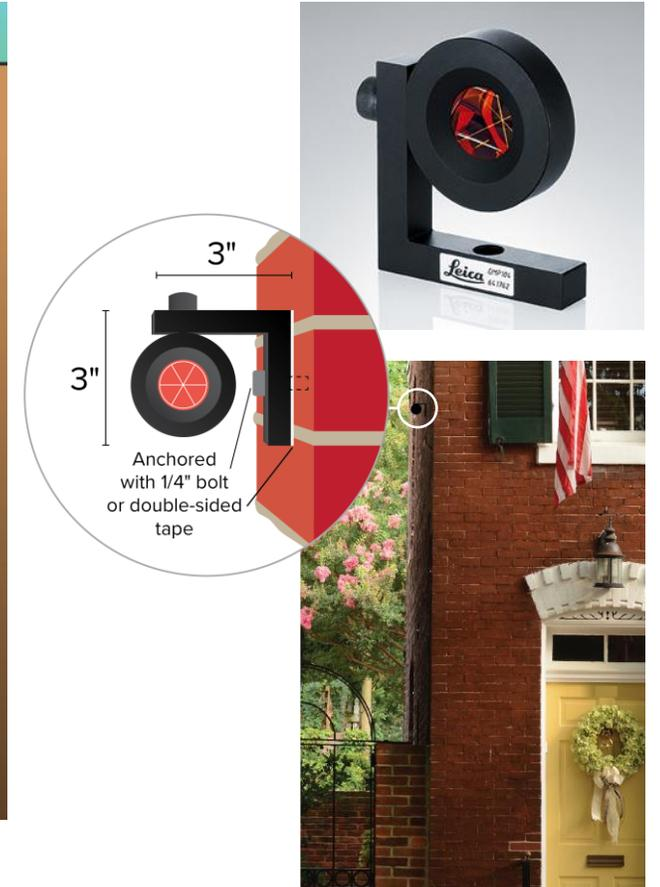
**Structural Monitoring Points** are passive devices used to survey a structure before, during, and after tunnel construction.
