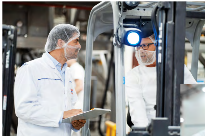
A blue light projected onto the floor in front of and behind the truck helps to avoid accidents.
