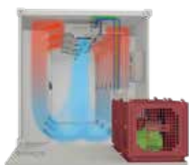
Fig. 1 Procedural principle for container cooling
